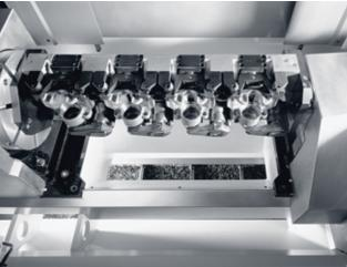
Large dimension rotary indexing tables and device bridges with torque technology enable stable and precise 4- and 5-axis machining. The alignment in the work space helps free chip fall.
