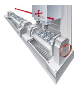
The machining centers with modular construction allow total freedom in the individual design of manufacturing processes.
